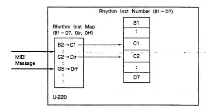
This setting determines how key numbers of an external MIDI instrument are related to the key numbers of the U-220 rhythm instrument. Each rhythm instrument map determines how each MIDI key number corresponds to each rhythm instrument number. Four rhythm instrument maps can be set. The Rx R.Inst Assign parameter determines which of these four maps is used. (page 48.)
