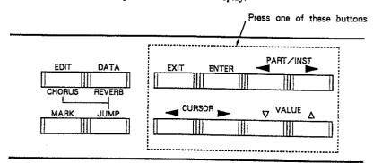
To move to the display you have marked, press JUMP and then press the button for which you have marked the desired display. (This procedure is also used to jump to the displays marked for EDIT and DATA.)
