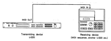
The dump function transmits data one way. In one-way transmission, the data is transmitted regardless of the condition of the receiving device.
