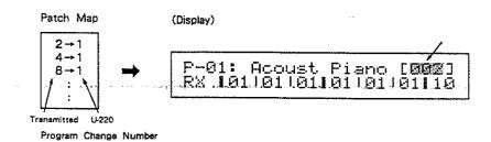
The lower line shows the reception channel and output for each part.
