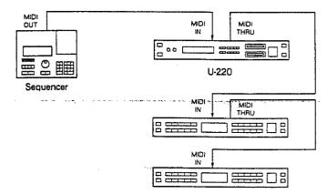
\* It is theoretically possible to use MIDI THRU to connect any number of devices. However three is about the practical limit. Running a MIDI signal through many THRUs can garble the transmitted data. If you need to connect more than three devices please use a MIDI Thru Box.
