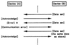
Device (B) rejects the data re - transmitted, and guits data transfer.
