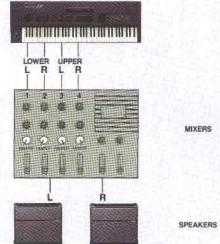
The sound signals from the Lower L and Lower R jacks are mixed by the mixer and come from this speaker.
