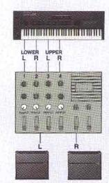
The sound signals from the Upper L and Lower L jacks are mixed by the mixer and come from this speaker
