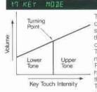
Two different tones can be changed by key touch: a stronger key touch produces the upper tone and a weaker one produces the lower tone. The value set for the patch memory factor 13 (Upper Split Point) is also used to determine how hard you have to press the key to change the tones The higher the value, the stronger you have to play
